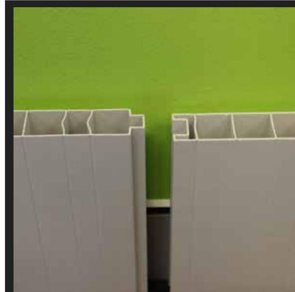
Easy fit tongue and groove join for fast installation and demounting. Pre-finished 300mm wide x 30mm thick pvc panels. (stocked lengths in selected increments from 2.4m to 6m.)
