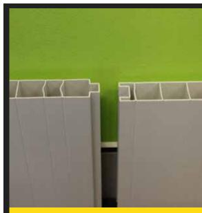
Easy fit tongue and groove join for fast installation and demounting. Pre-finished 300mm wide x 30mm thick pvc panels. (stocked lengths in selected increments from 2.4m to 6m.)
